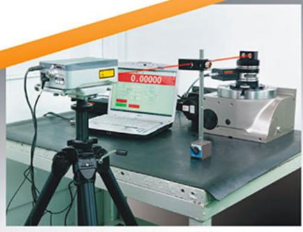
Renishaw laser instrument is applied for inspecting indexing accuracy.
